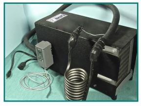
The digital readout displays the present temperature when the thermostat is in the water.
