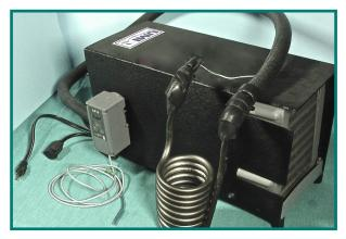
The digital readout displays the present temperature when the thermostat is in the water.
