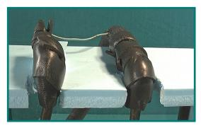
Cut a 6" section of the styrofoam lid for the wrapped section of coils to rest on. Cut two wedges to stabilize the coils. If the model comes with an attached metal plate, rest this plate on top of the lid.
